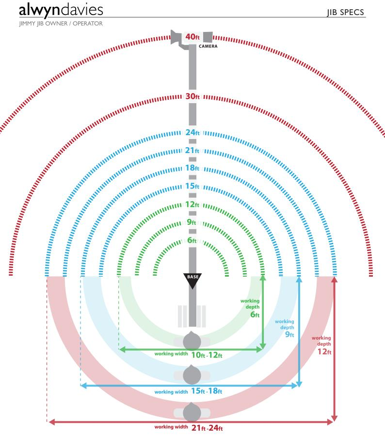
180 Degree arc of operation for the front of the Jib arm requires 180 Degree arc of footprint (shaded area) for the rear length of the Jib plus space for the Operator. Similarly, a 90° front arc requires a 90° rear as a 360° arc needs a 360° footprint.
